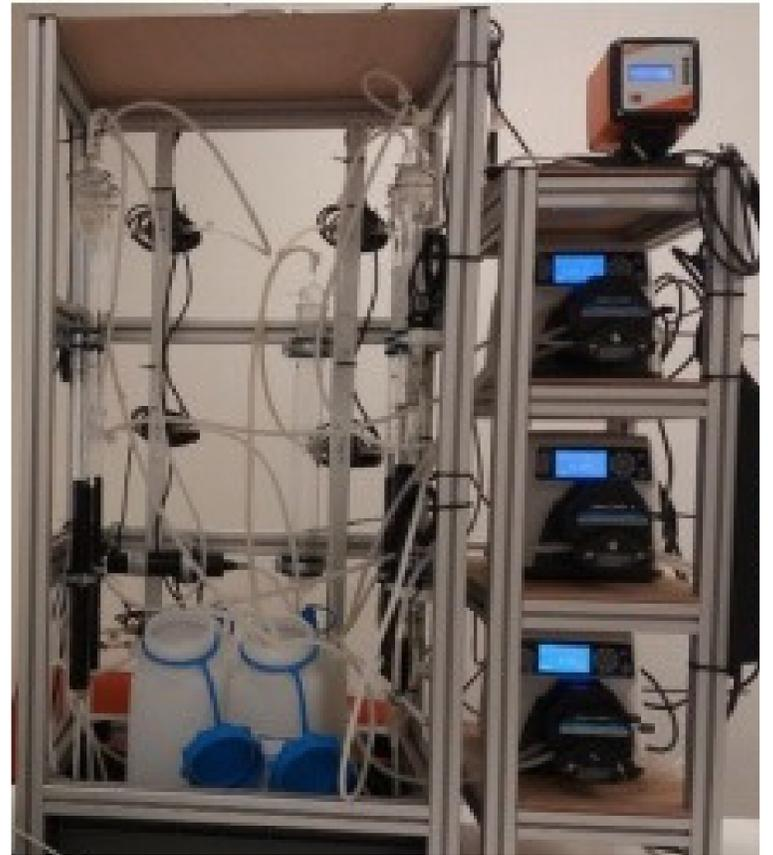
Figure 1 - Completed Ion Exchange lab set up
