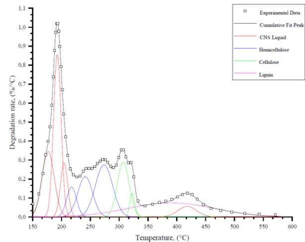
**Figure 2.** Gaussian deconvolution of DTG curve from thermogravimetric analyses performed under high-resolution approach (initial heating rate: 30 °C/min; resolution: 5; sensitivity: 1.0) for raw cashew nut shell. The graph shows the deconvoluted peaks for hemicellulose (blue), cellulose (green), lignin (pink) and cashew nut shell liquid (red). Temperature range selected from 150 to 600 °C. Coefficient of determination ( $r^2$ ): 0.9994.
