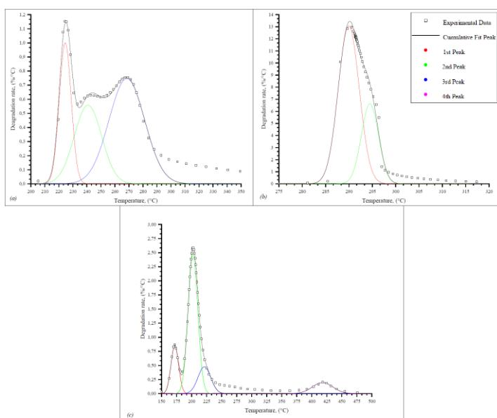
**Figure 1.** Gaussian deconvolution of DTG curves from thermogravimetric analyses performed under high resolution approach (initial heating rate of 30 °C/min; sensitivity 1.0; and resolution 5.0) for (a) xylan, (b) microcrystalline cellulose (MCC) and (c) cashew nut shell liquid (CNSL). Coefficient of determination ( $r^2$ ): a) 0.961, b) 0.994 and c) 0.997.
