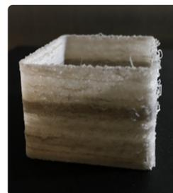
Figure 6: Inadequate hollow square
