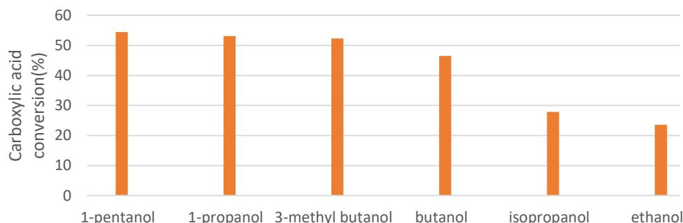
Figure 3. Extent of esterification of the bio-oil at 40 °C using different types of alcohol and 5% of catalyst.
