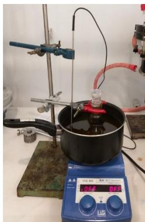
Figure 2. Batch reactor used in the experiments.
