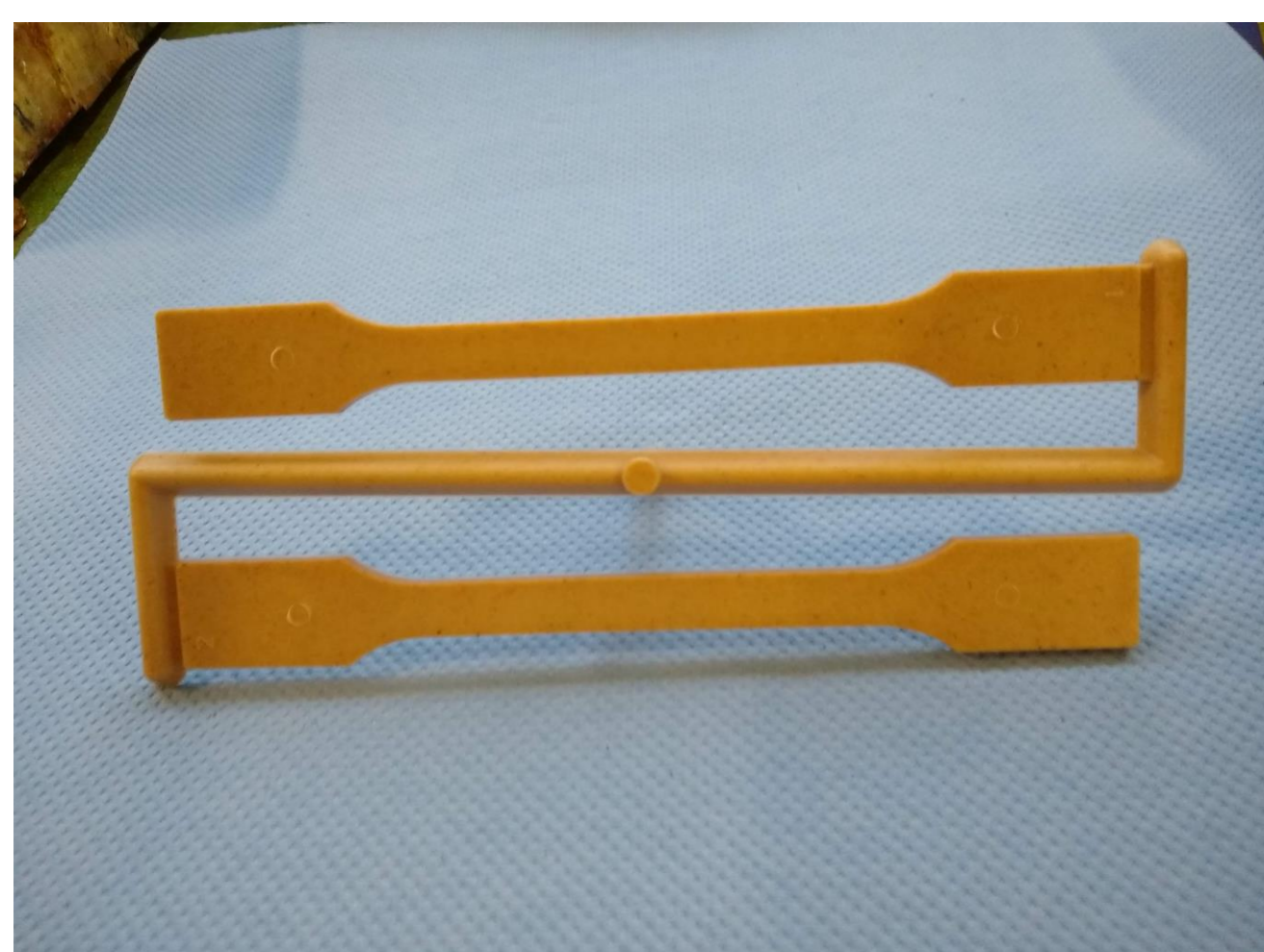
Figure 2- Samples of PHBV with wood fibre moulded by injection moulding for mechanical properties tests.
