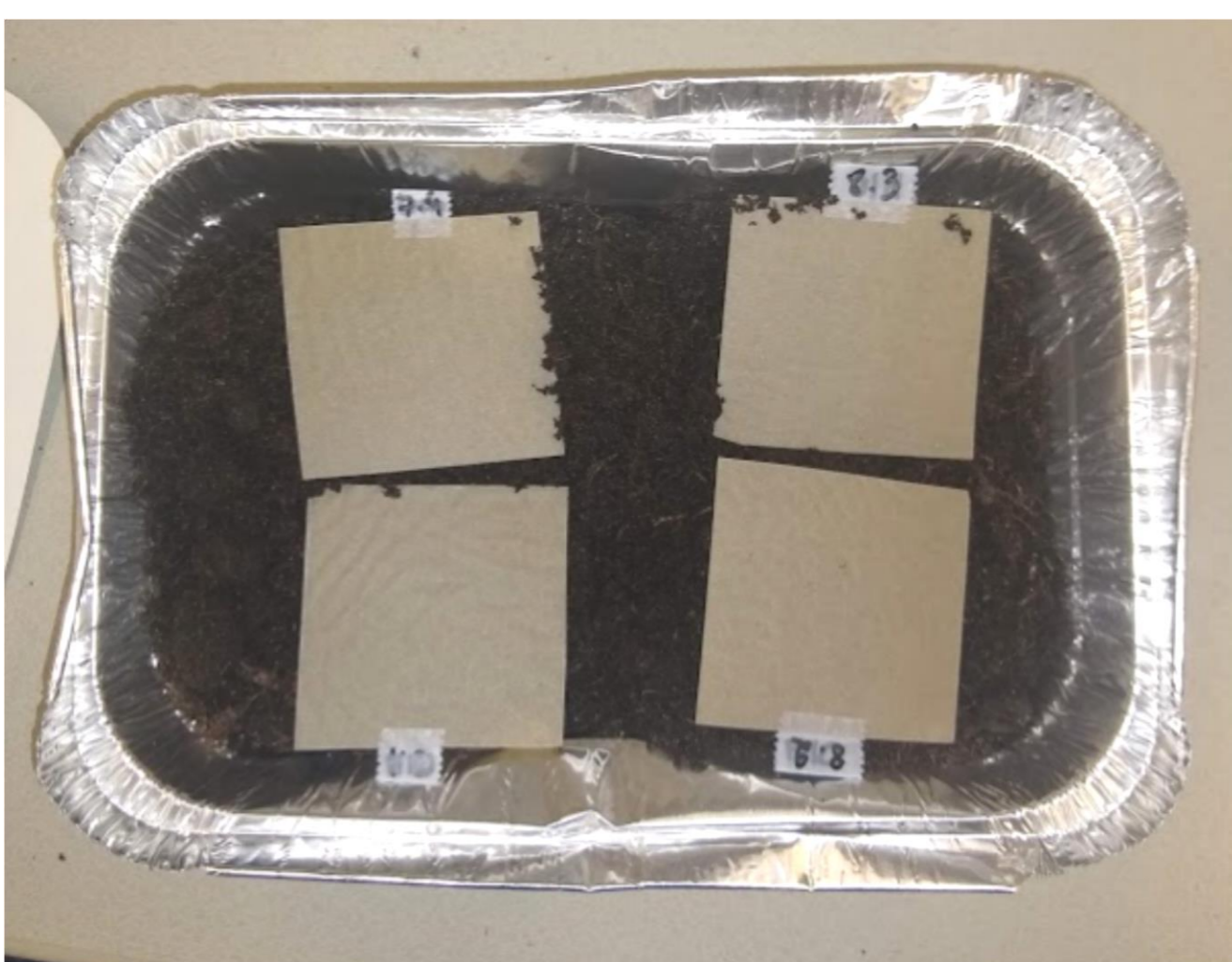
Figure 1- Samples of PHBV with hemp fibre moulded by compression moulding buried in soil for starting the biodegradation process.
