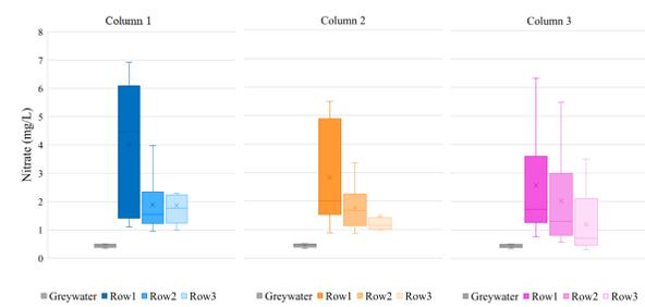
Figure 6. Nitrate concentration for each module from each experimental column.
