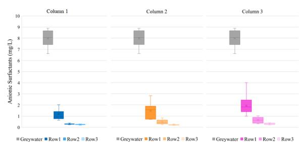
Figure 3. Anionic Surfactants concentration for each module from each experimental column.
