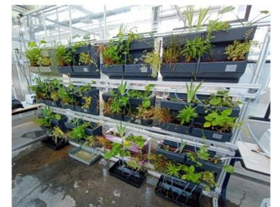
Figure 2. Green wall/vertical wetland setup used to conduct the experiments.
