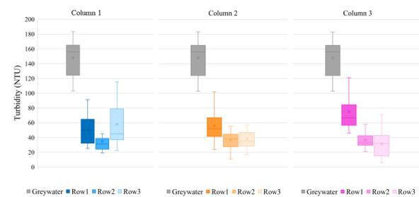
Figure 9. Turbidity levels for each module from each experimental column.
