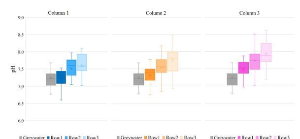
Figure 8. pH levels for each module from each experimental column.
