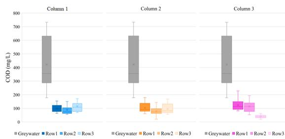
Figure 4. COD concentration for each module from each experimental column.
