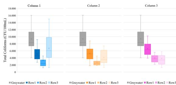
Figure 10. Total Coliform count for each module from each experimental column.
