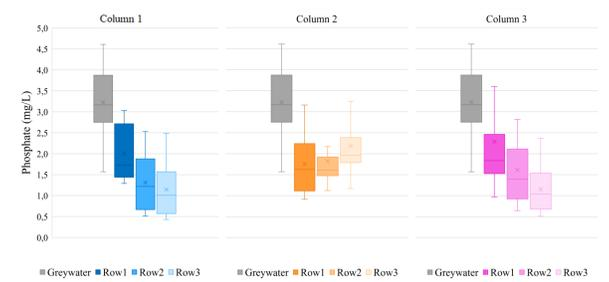
Figure 5. Phosphate concentration for each module from each experimental column.
