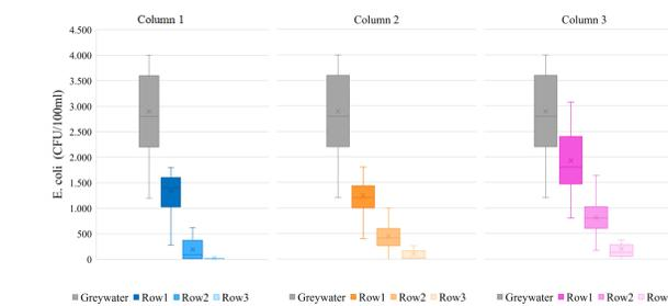
Figure 11. Faecal Coliform count for each module from each experimental column.
