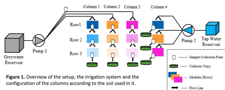
Figure 1. Overview of the setup, the irrigation system and the configuration of the columns according to the soil used in it.
