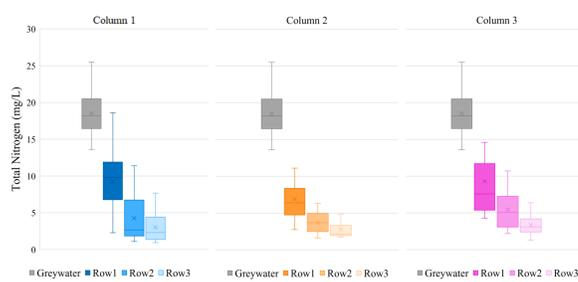
Figure 7. Total N concentration for each module from each experimental column.
