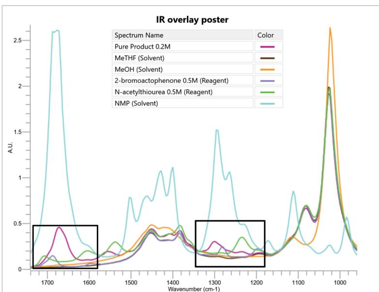
Figure 6. Spectra overlay with reagents, solvents and product
