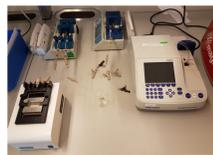
Figure 3. Labtrix set-up with in-line UV-VIS
