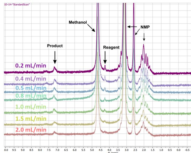
Figure 7. In-line H-NMR measurements of a reaction at 0.5 M at different flow rates
