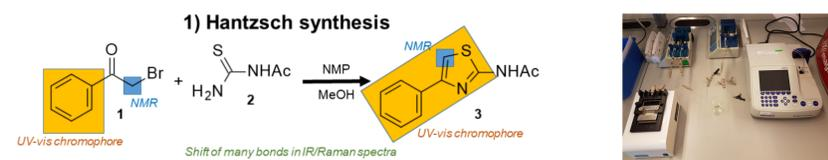
Figure 2. Hantzsch Reaction scheme. 1: 2-bromoacetophenone; 2: N-acetylthiourea; 3: 2-acetamido-4-phenylthiazole
