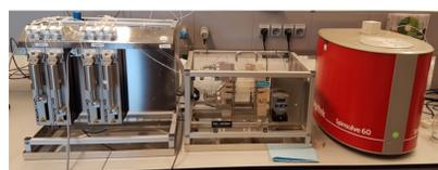
Figure 4. Kiloflow set-up with in-line H-NMR
