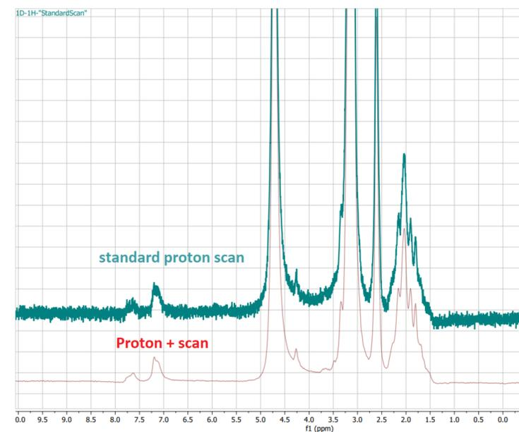
Figure 8. Comparison between an H-NMR measurement done with the standard proton scan and one done with the proton + scan. Both measurements were done with reagents at 0.5M and 0.5 ml min
