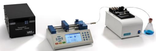
Fig. 4: Labtrix Start flow reactor set up.
