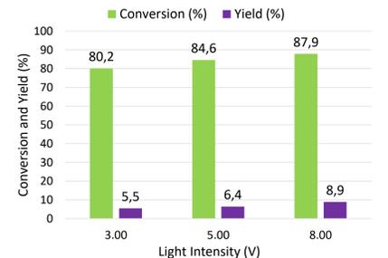
Fig. 7: Effect of different light intensities on conversion and yield.
