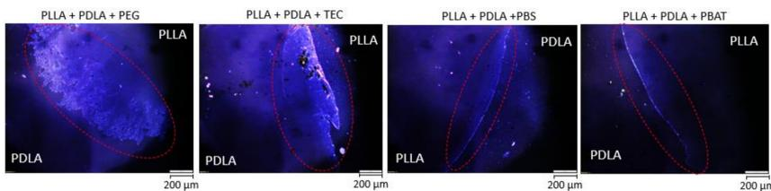
Figure 2. Effect of each plasticizer/polymer on the stereocomplexation of PLLA and PDLA after 10 min of contact in the polarized light microscope with hot stage
