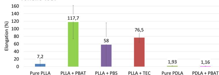
Figure 4. Elongation at break of horizontally cut samples from a single wall 3D printed object.
