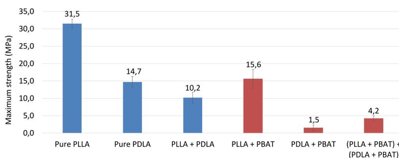
Figure 5. Maximum strength of vertically cut samples from two walls 3D alternated printed. Samples of pure PLLA or PDLA and PLA/PBAT has been studied.
