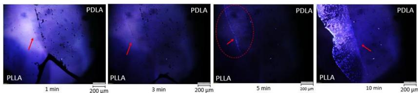
Figure 1. PLLA-PDLA behavior under polarized light microscope upon heating the sample at 200 °C for 10 minutes
