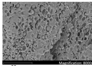
Figure 3. SEM result of two different phases in blend of PDLA + PBAT
